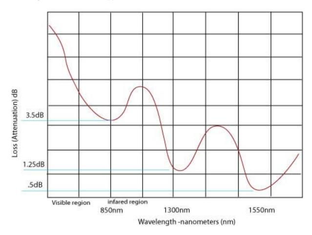
850nm - 3-4dB of loss/km. The least expensive transmitting device. Found on lower speed, shorter distant applications such as CCTV, Fire Alarm communication devices. ( LED) Used with Mulit-Mode fibers
